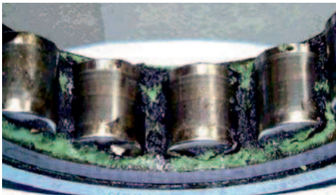
Lubricant degradation caused by electrical discharge currents
